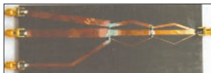
▲ Fig. 4 Photograph of the fabricated dual-frequency unequal power divider.
