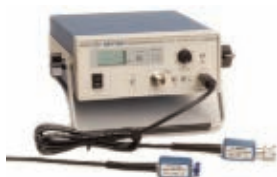
RF & Microwave Power Meter 100 KHz to 40 GHz
